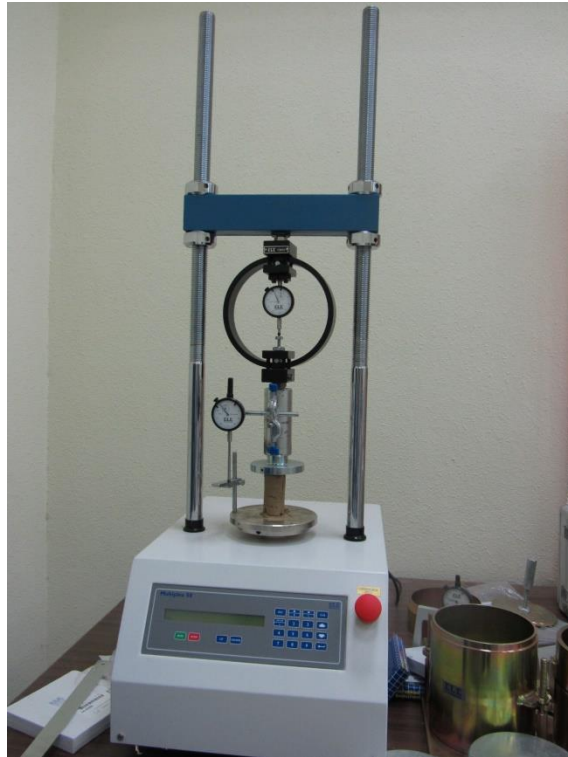
Fig(2) Unconfined compression Test
