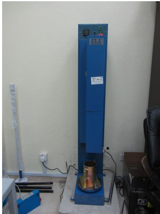
Fig (6) Automatic Soil Compactor
