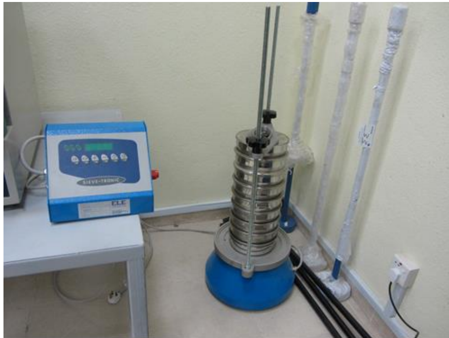
Fig. (10) Sieve Shaker (Soil Grain Size Analysis)
