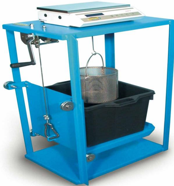
Fig (8) Specific Gravity & Water Absorption
