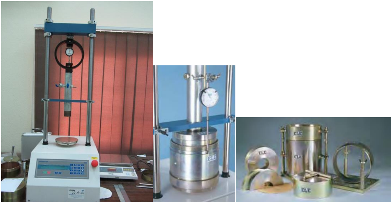
Fig. (11) California Bearing Ratio
