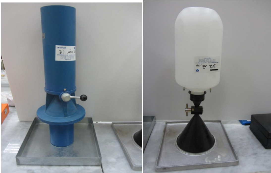
Fig (7) Insitu Field Density Sand Cone Method
