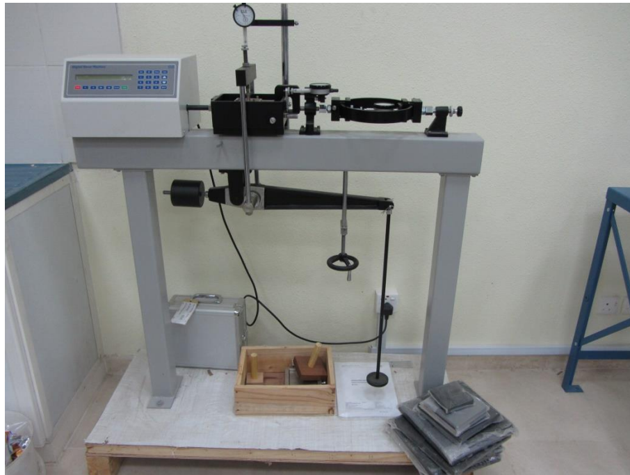
Fig (3) Shear Box Test
