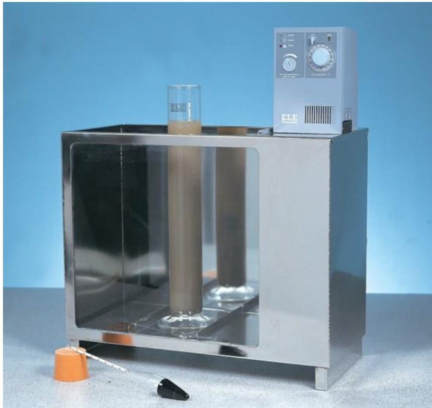
Fig. (12) Hydrometer Test (Grain Size Analysis)
