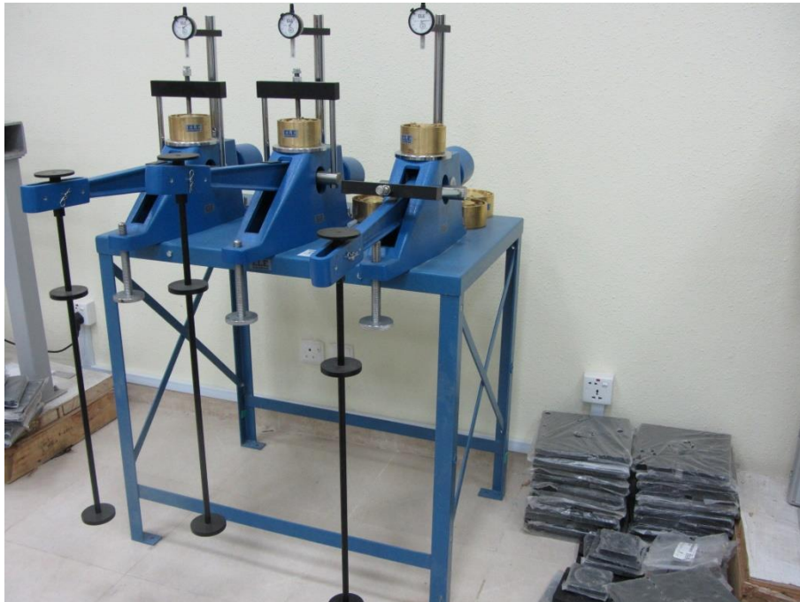
Fig.(5) Oedometer, Consolidation of soil
