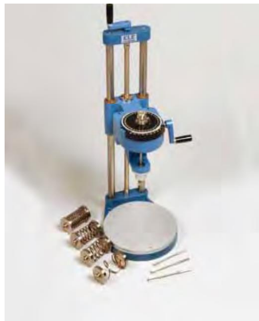
Fig. (13) Laboratory Vane Shear Apparatus
